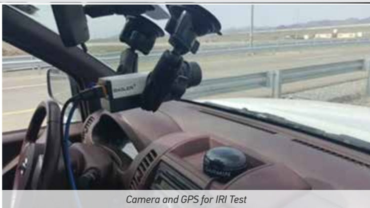
IRI machine mounted on CCC Pickup
